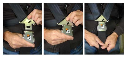
8. Tighten Shoulder Straps to adjust seating position for smaller pilots
