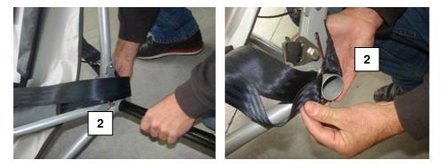
3. Ensure the straps cross over and tension in place N.B. Tensioners used when fitting to shadow seat or early model karts
