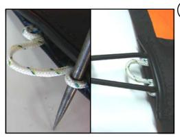
Thread the bungee through the loops of the white cord from the back, you may need to open the loops with a tapered tool.
