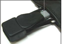
NB. The blokart<sup>®</sup> batten retainer cap allows for personal tuning options. Lengthen the bungee tails behind the knots to increase the batten tension.
